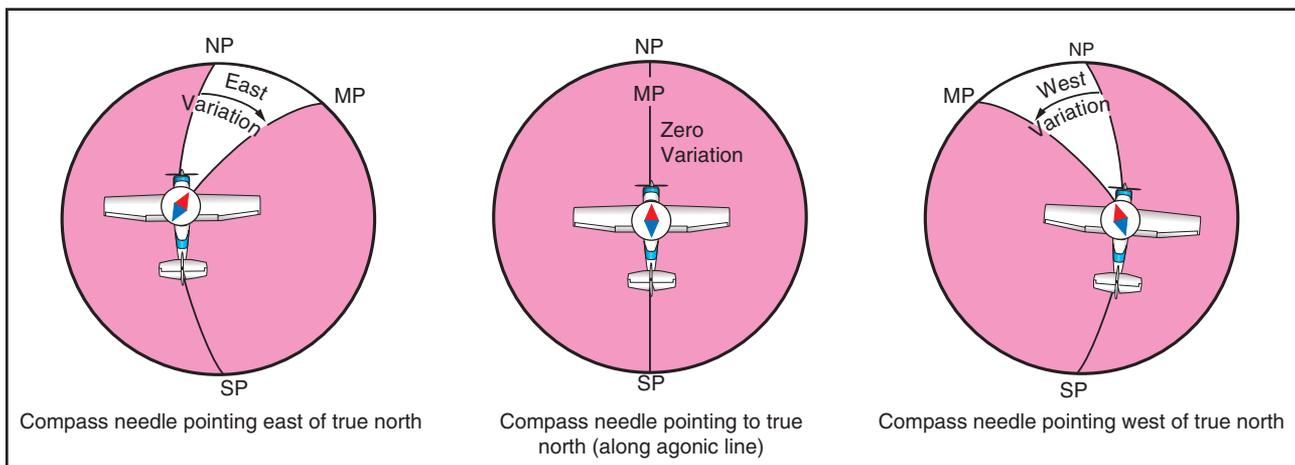
Figure 14-8. Effect of variation on the compass.
